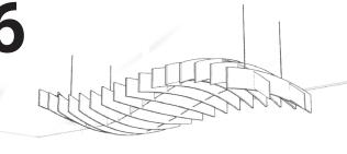
Thread the mount caps onto the cables, followed by the cable clips. Then screw the assembled cables into the fixed ceiling mounts.
