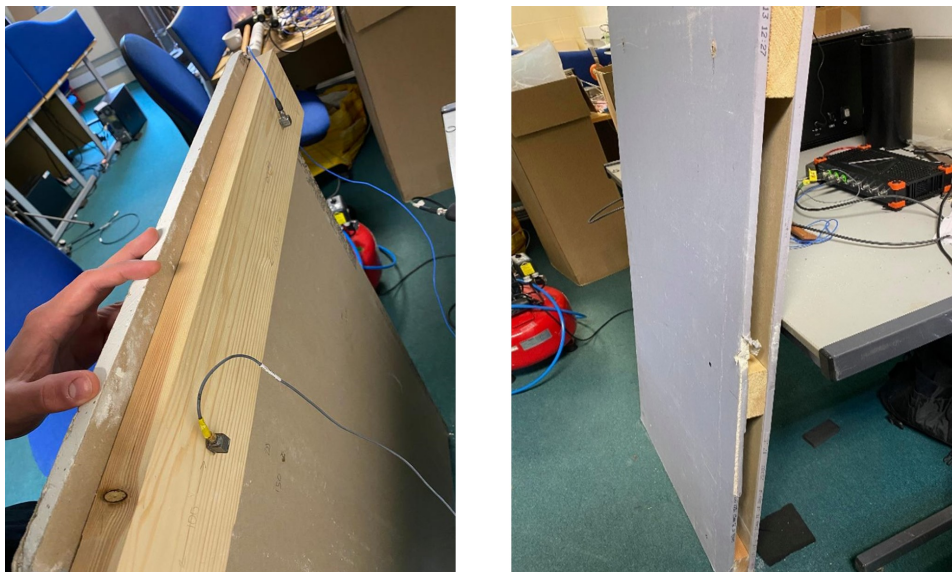
Figure 6: The left picture shows plasterboard screwed into a timber beam, the right picture the full system of plasterboard - beam - plasterboard.
