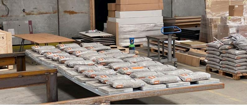
The strength of the fence (modules and posts) is determined by testing until breakage.
