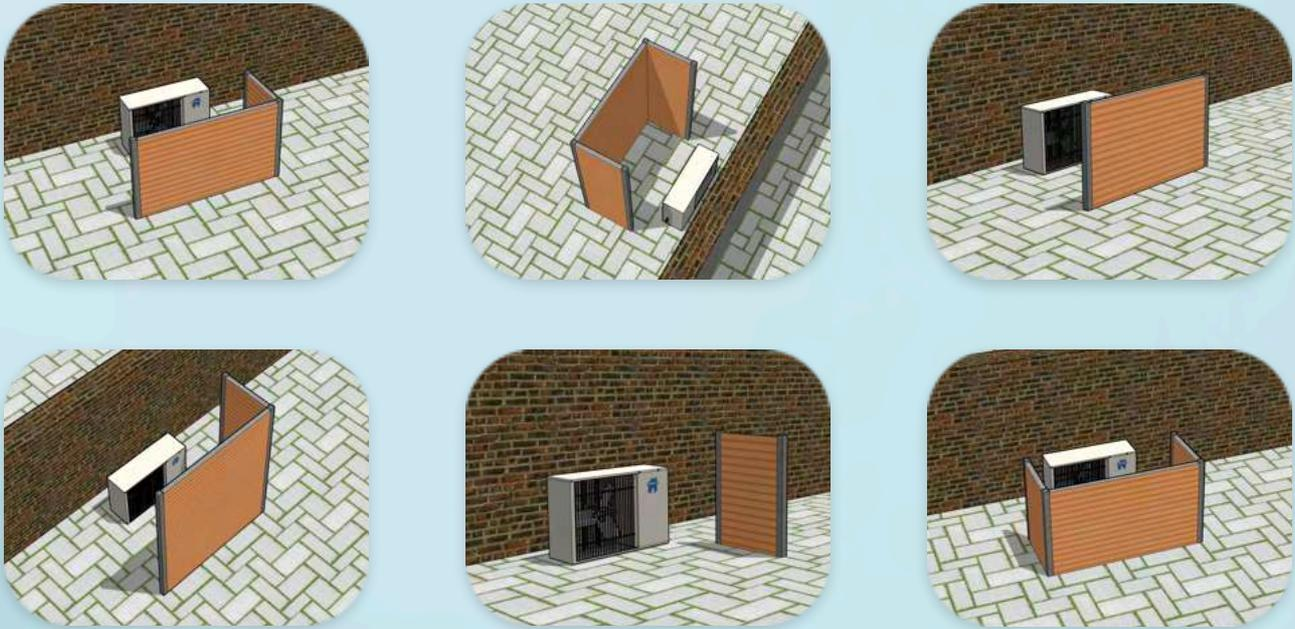
Figure 10 - Configuration Group B examples. *Top Left* - 1m L-shape (Multiple Panel). *Top Middle* - 2m U-shape (Multiple Panel). *Top Right* - 1m Front. *Bottom left* - 2m L-shape (Multiple Panel). *Bottom Middle* - 1m Side. *Bottom Right* - 1m U-shape (Multiple Panel)
