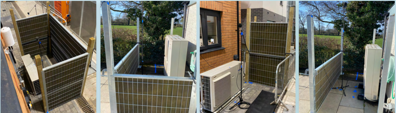
Figure 2 - Left - U-shape (2m) configuration laboratory. Left Center - L-shape (1m) configuration outdoor. Right Centre - Side Panel (2m) configuration laboratory. Right - Front Panel (1m) configuration outdoor.
