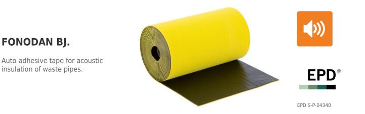
FONODAN BJ is a two layer product made of a self-adhesive high density bitumen membrane thermally bonded to a cross-linked polyethylene. FONODAN BJ acoustically works providing the acoustic mass of the tube body and removing resonant frequencies.
