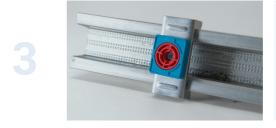
MuteClip metal furring channels clip into the MuteClip claws and will suspend your new acoustic board layers away from the existing structure. It also provides space for acoustic mineral wool.
