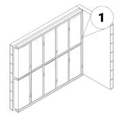
Measure, mark and screw MuteClips directly to the stud or brick.
