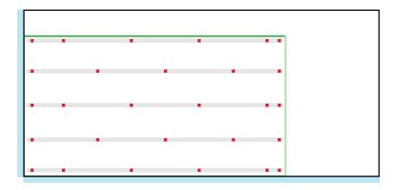
The red dots show where MuteClips need to be fixed to your wall. Through the clips, metal furring channels will be placed. Use the sheet opposite to create your own template and the instructions over leaf for detailed installation method.
