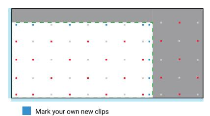
Finally, add an extra MuteClip to the end of every row down the right hand side. Mark these <100mm away from the wall perimeter. It is fine for this clip to be closer to the previous fixing than normal.
