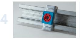
MuteClips and metal furring channels suspend your new soundproofing boards away from the existing wall. These decouple the system and provide the best reduction for space used.
