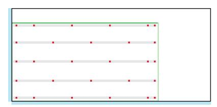
The red dots show where MuteClips need to be fixed to your wall. Through the clips, metal furring channels will be placed. Use the sheet opposite to create your own template and the instructions over leaf for detailed installation method.
