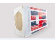
Acoustic mineral wool of 60kg/m³ or more is best for ceilings. The high mass gives it acoustic properties thermal insulation doesn't have.
